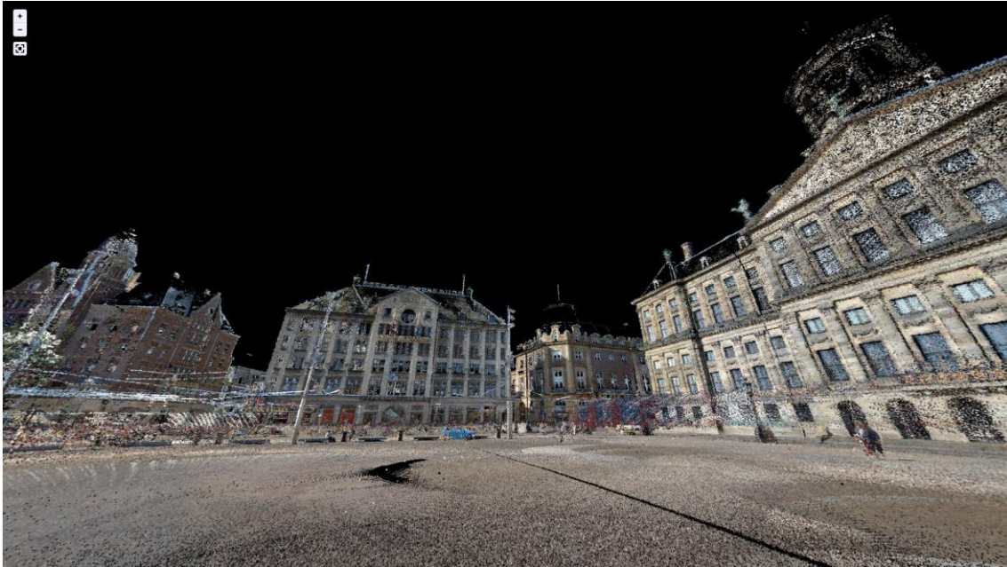
Figure 50 – Mobile LiDAR scan of the same area (Cyclomedia, 2018)
