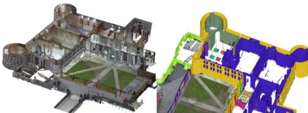
Figure 24 – 3D point cloud representation (left) and a 3D semantic representation (right) (Source: Poux, 2019)
