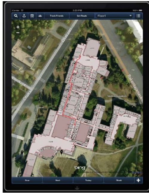
Figure 2.1: Nikander et al. (2013)’s prototype application with an indoor floor plan overlaying outdoor satellite imagery
