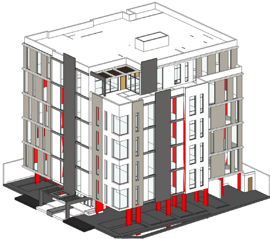
FIG. 10.3 3D IFC model of a real-world complex building
