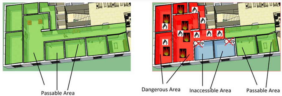
FIG. 2.25 Union of topographic spaces to represent dangerous areas.
