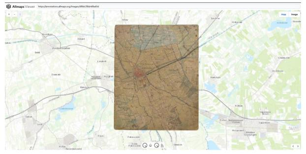
Figure 4 Displaying the result of georeferencing tin the Allmaps Viewer.
