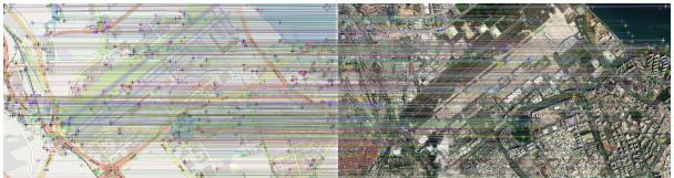
Figure 37 Image from GitHub repository of Lan et al., showing found features between OpenStreetMap(left) and satellite image (right). (Lan et al., 2021)
