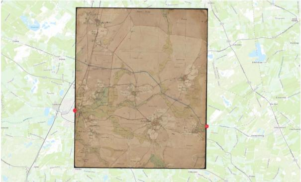
Figure 51 Same map as in previous figure, but now with correct georeferencing. Red dots mark the locations of the arrows from the previous image.
