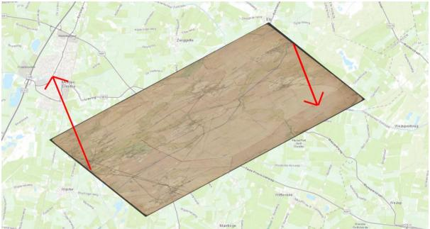
Figure 50 Result of georeferencing is in the correct location, the correct scale but highly skewed and squashed. Red arrows show where the map locations should have been georeferenced to.
