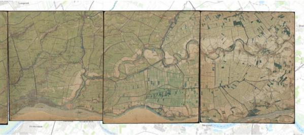
Figure 61 Georeferenced results forming an interconnected sequence that lines up accurately.
