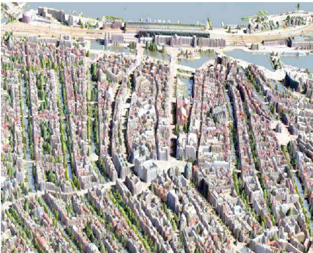
Figure 2.12 Aerial image of the centre of Amsterdam draped on top of unfiltered AHN (source: AGI, Ministry of Transport, Public Works and Water Management)
