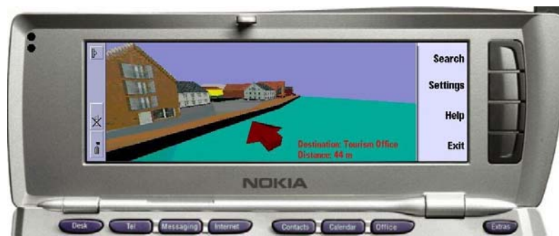
Figure 3: 3D models with Nokia GL on the Communicator 9210 as one result of the TellMaris project (IST-2000-28249, http://www.tellmaris.com ). © Nokia Research
