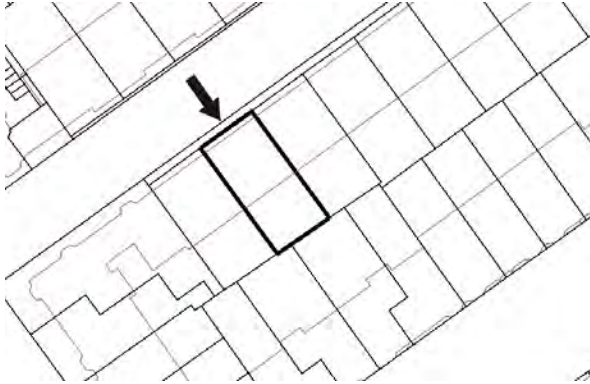
Figure 3.6: The cadastral map of the apartment complex in figure 3.4. The parcel in question has been drawn with a thicker line-style. The front of the building is indicated with an arrow. Note that the parcel is larger than the footprint of the building, since the parcels also includes a garden ('twin' in drawing of deed of division).
