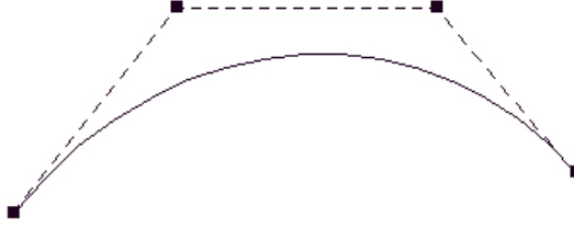
Figure 2.1: A cubic (degree 3) Bézier curve
