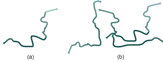
Figure 3.6: Vague line objects: (a) a vague line, (b) a vague multiline.
