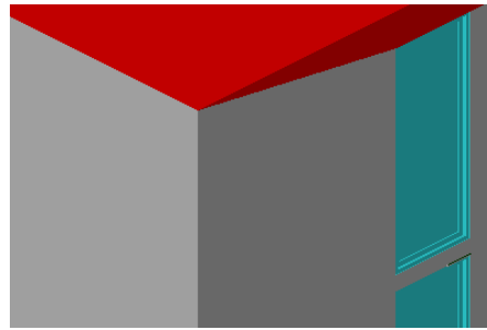
(B) Output CityGML model, the border edges between the vertical roof and wall faces are removed
