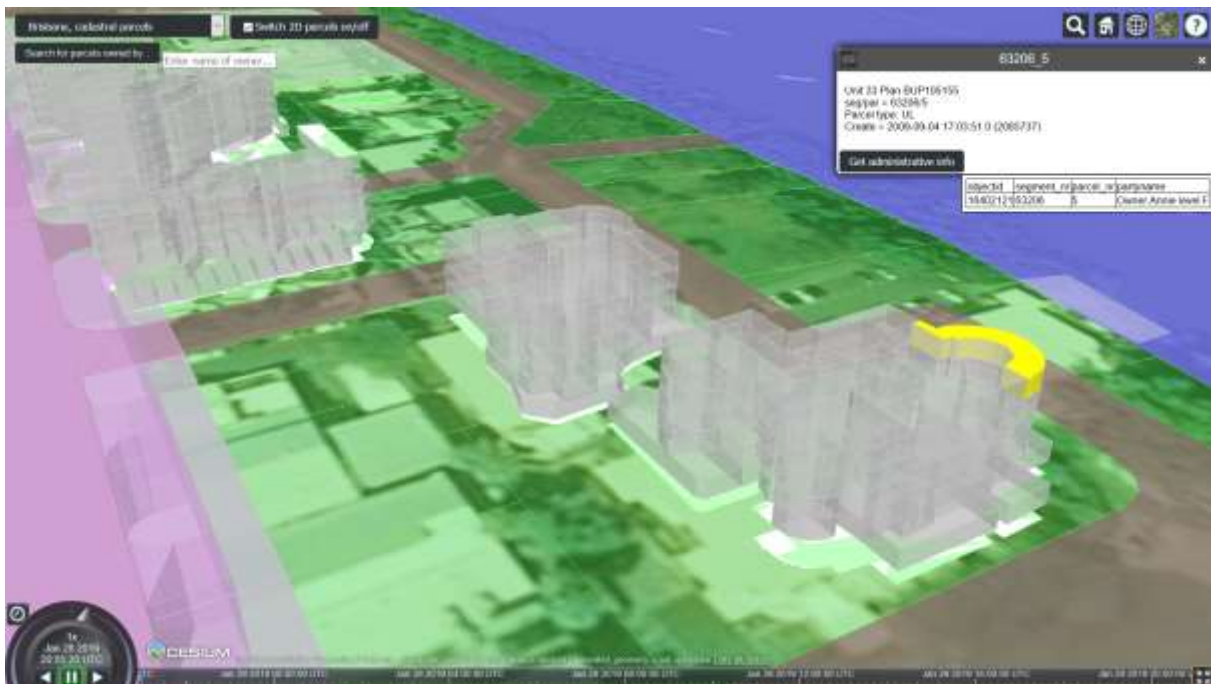
Figure 1. Web-based 3D cadastral client showing the selection of an apartment (yellow highlight, on the left side of the image)
