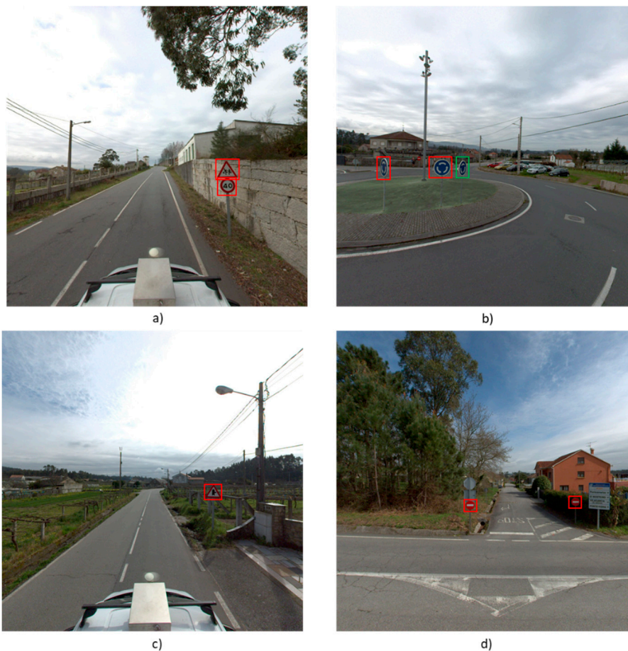
Figure 6. TSs detected: case study 1 with frontal cube-image (a), and with lateral cube-image (b), case study 2 with frontal cube-image (c) and with lateral cube-image (d). Detected TSs remarked in red boxes and filtered TSs remarked in green boxes.
