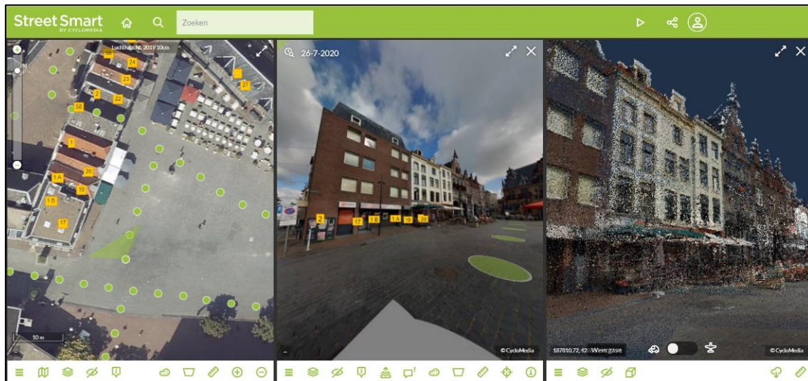
Figure 3.3: The Cyclomedia web viewer showing (from left to right) an aerial photo from above, an aerial photo from street level and a point cloud of the Market in Nijmegen (Cyclomedia, 2020).
