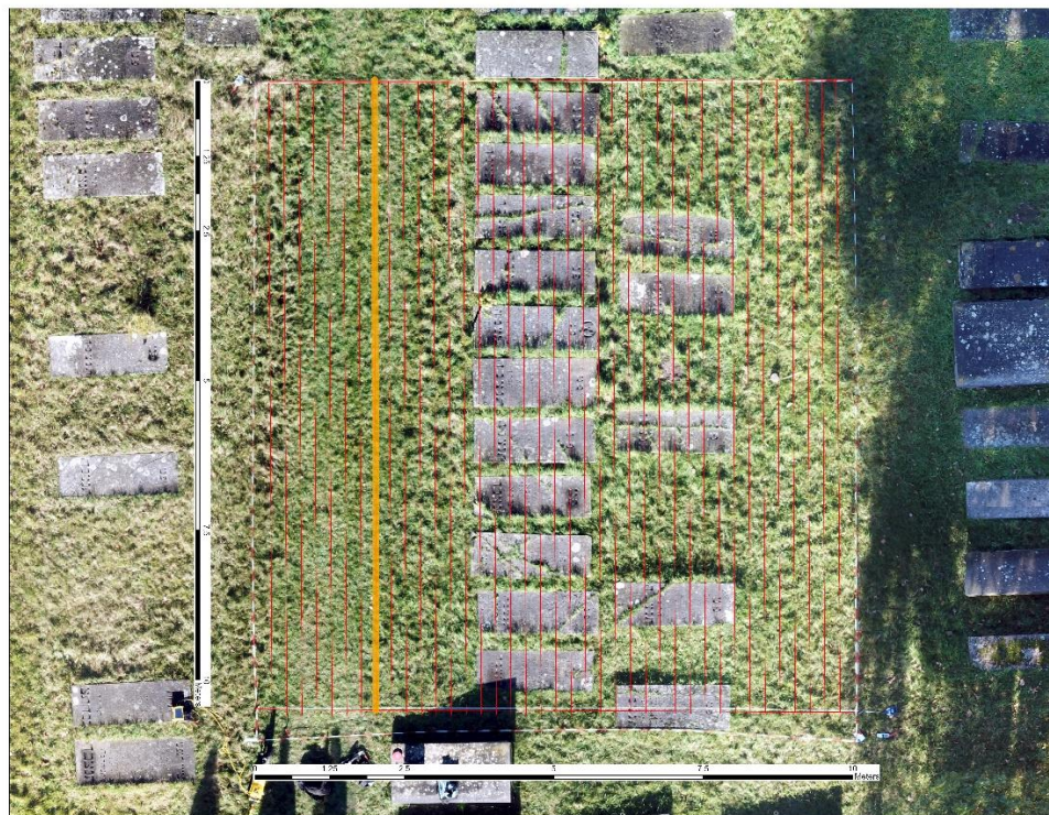
Figure 16: Orthomosaic of area AB1 with overlaid GPR grid and highlighted line #32 (Author).
