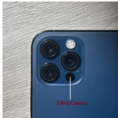
Figure 3.2.: LiDAR sensor of iPhone 12 pro
