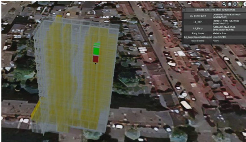
Figure 16. Enriched BIM/IFC model visualised in an online visualisation platform (Broekhuizen, 2022)
