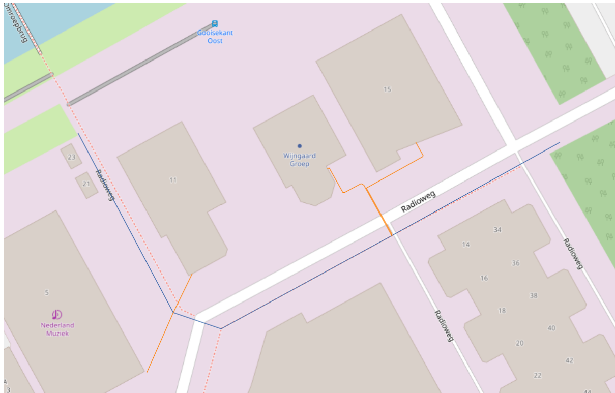
Figure 33. Selected pipe segments from the sewerage network in Almere. Blue: main sewerage pipes, orange: home connections
