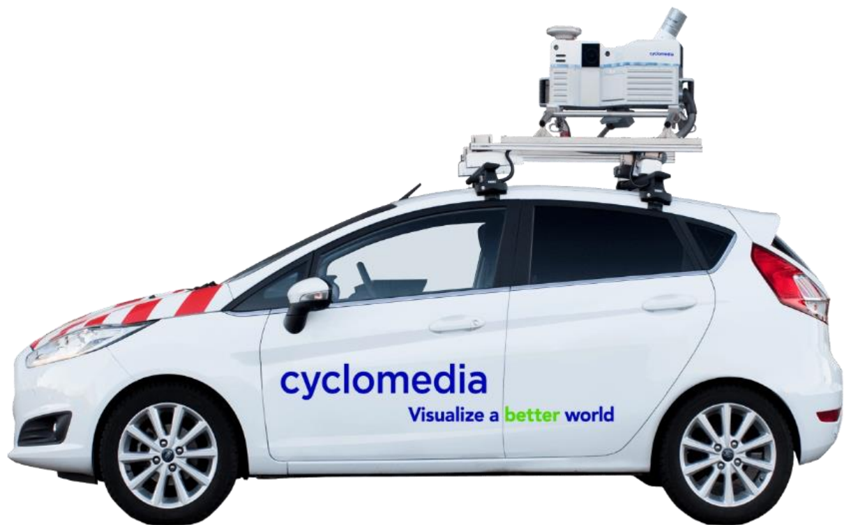
Figure 35: Cyclomedia's mobile data acquisition vehicle (source: Cyclomedia).
