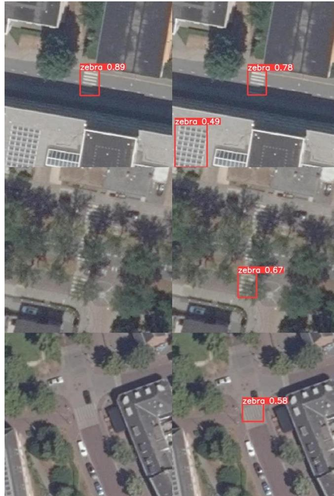
**FIGURE 20: PREDICTIONS COMPARISON BETWEEN THE ORIGINAL (LEFT IMAGES) AND THE FINE-TUNED (RIGHT IMAGES) MODELS.**
