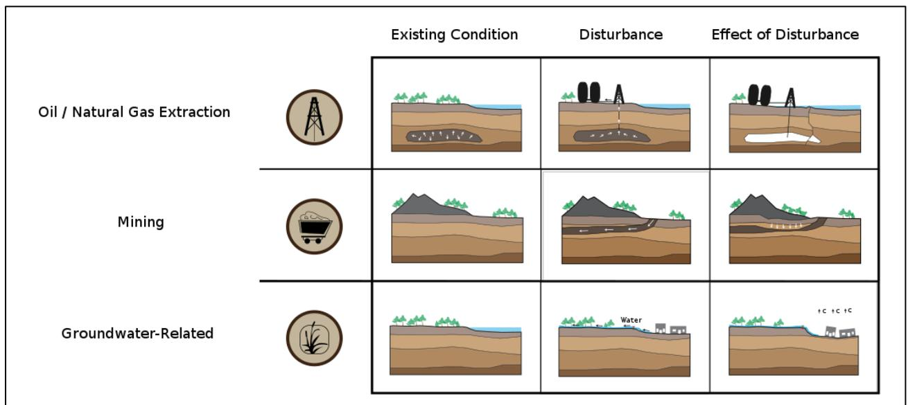
Figure 1: Examples of types of subsidence and their causes (source: (Petty, 2011))
