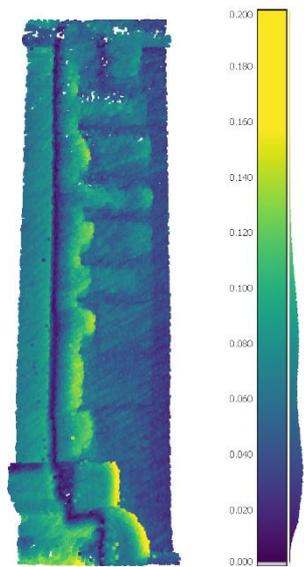
**Figure 4 - Corner section point-cloud coloured based on the distance between the ZEB-Horizon and iPhone model**
