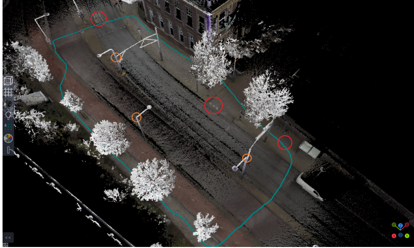
Figure 4.6.: Calibration Data: Ground (red), Height (orange) control points and Trajectory (green).
