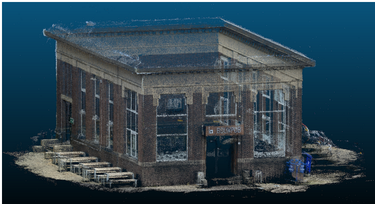
Figure 1.2.: Using photogrammetry technique to reconstruct a pub with 102 images
