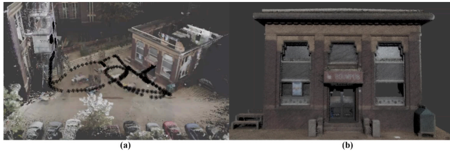
Fig. 13. Blender-Based Integration of Point Clouds and 3D Gaussian Splatting. (a) Overview of the 3D Reconstruction in Blender; (b) Result of Blender-Based splatting.
