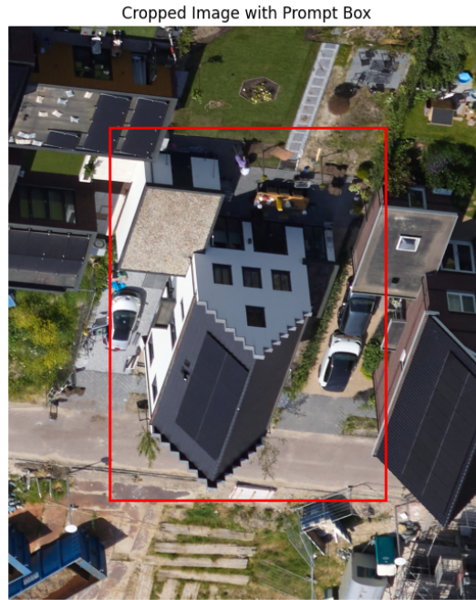
Figure 4.3.: Reprojected bounding box (red square, also used as the box prompt) within the cropped image. The image is the result of adding a 250-pixel buffer on each side of the original bounding box.
