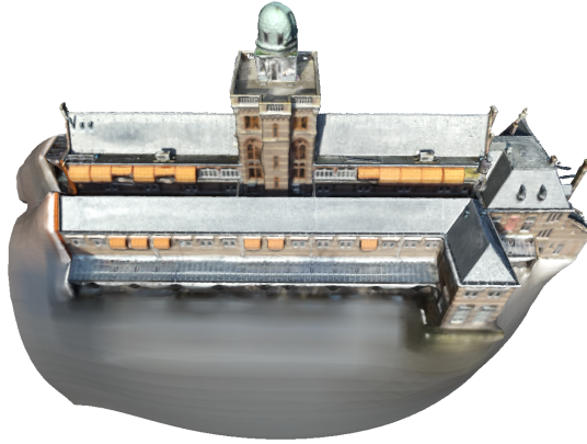
Figure 6.3.: Mesh from the SAM kernel entropy method with threshold 0.3, showing the underside of the mesh clearly as an artifact
