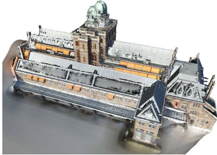
Figure 4.6.: Misalignment of ground truth mesh and 0.7 Image-based Canny Edge Entropy thresholded mesh.
