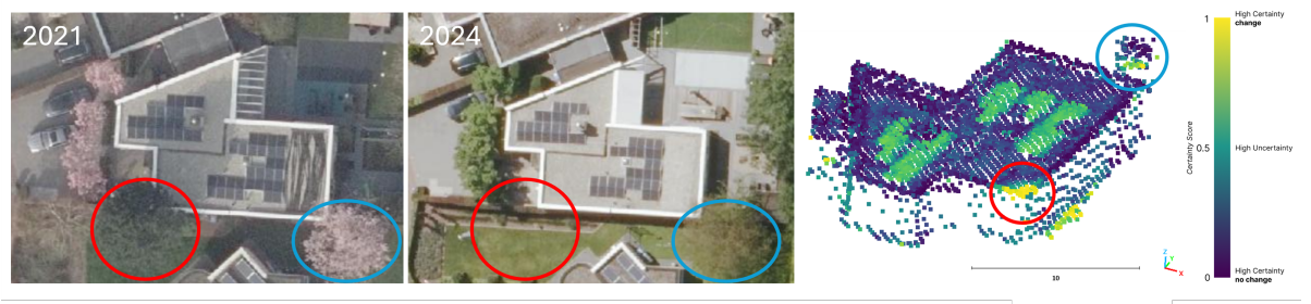
Figure D.4.: False change detection due to tree points within building-labelled raster cells (blue circle). In addition, removed opaque vegetation between epochs results in regions consistently labelled as changed due to persistent occlusion in the reference point cloud dataset (red circle). Orthophotos from 2021 and 2024 are provided for context, source: Beeldmateriaal Nederland .
