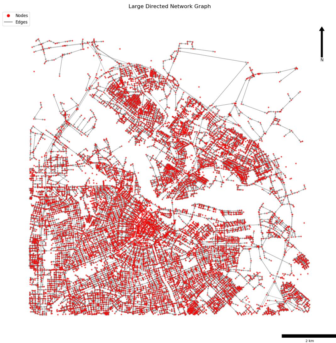
Figure 3.2.: Graph structure of the road network built from spatial data using `networkx.DiGraph` EPSG:28992.
