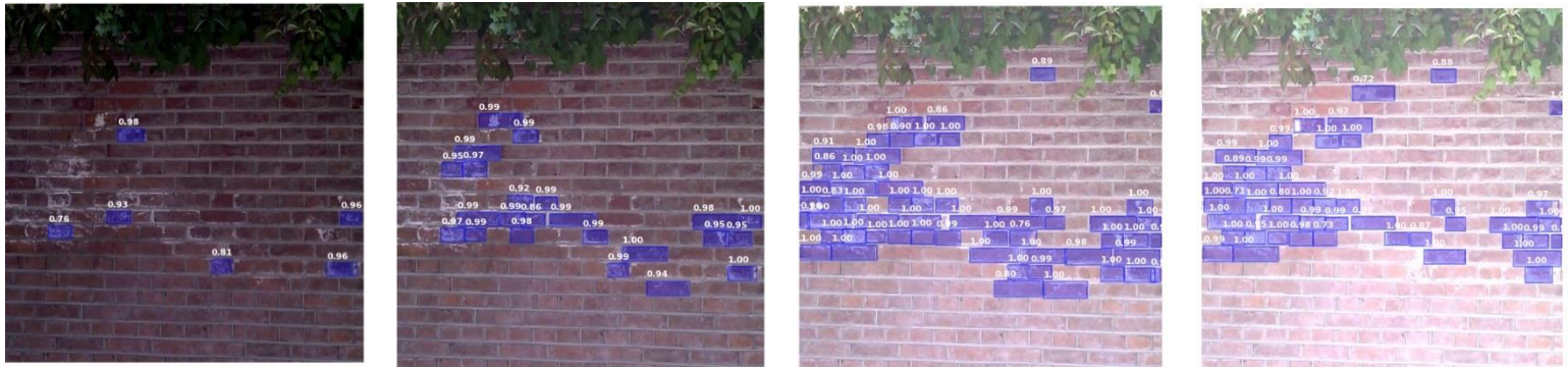
Figure 63 Prediction comparisons for brightness/contrast augmentation ( \pm 10\% , \pm 20\% ) versus the baseline
