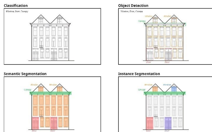
Figure 12 Illustration of the primary computer vision tasks: (a) image-level classification, (b) bounding-box object detection, (c) pixel-wise semantic segmentation, and (d) instance-level segmentation. Adapted and illustrated based on Liu et al. (2020).
