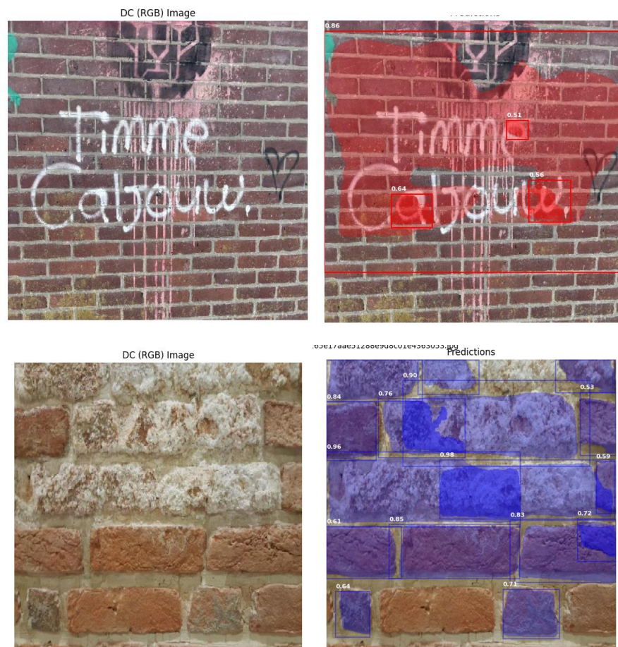
Figure 44 Efflorescence and Graffiti predictions results with confidence scores (Epoch 60) (1) Original graffiti image. (2) Graffiti prediction. (3) Original Image: (4) Efflorescence prediction.
