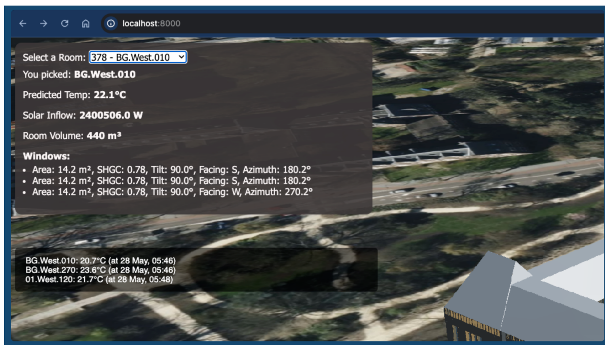
Figure 3.4: Web-based application interface for visualizing IFC-derived building model and displaying predicted indoor temperature results for user-selected rooms
