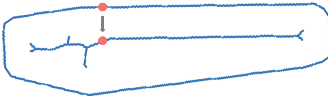
Figure 2.6.: A full shift from building outline to medial axis
