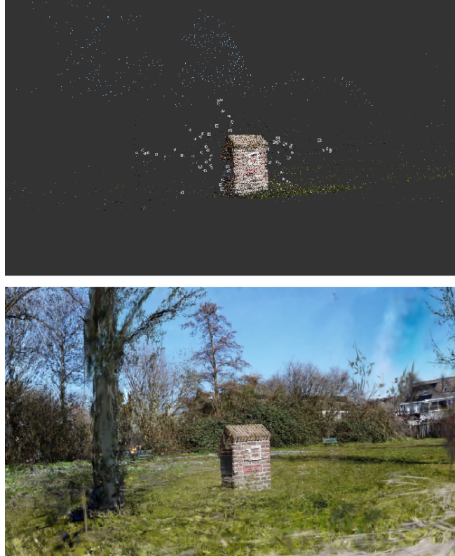
Figure 3.7.: The SfM point cloud (and camera positions) and Gaussian Splatting generated and viewed in Postshot.
