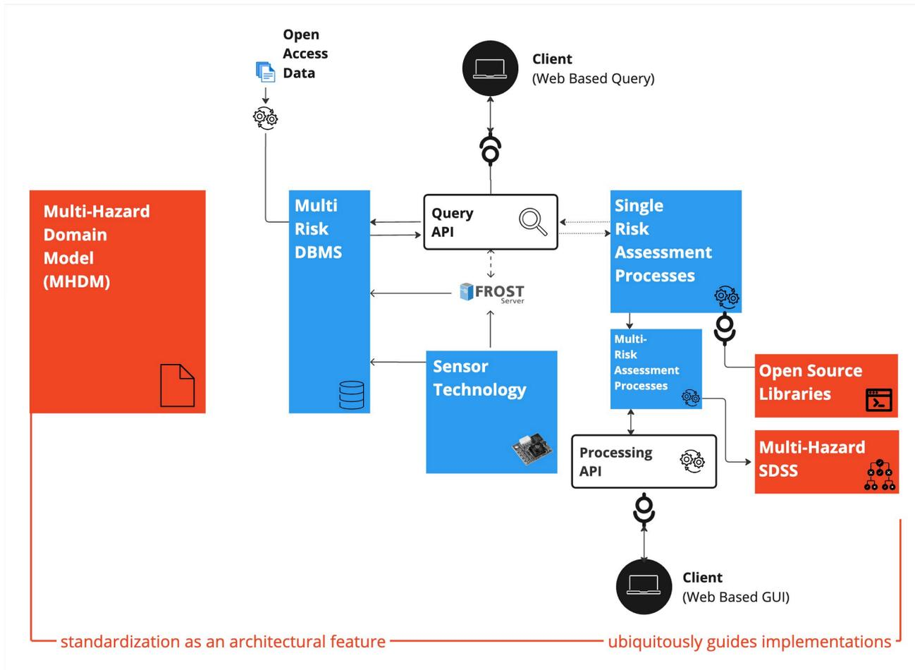
Fig. 1. Simplified architectural schema showing the components of a multi-hazard SDSS.
