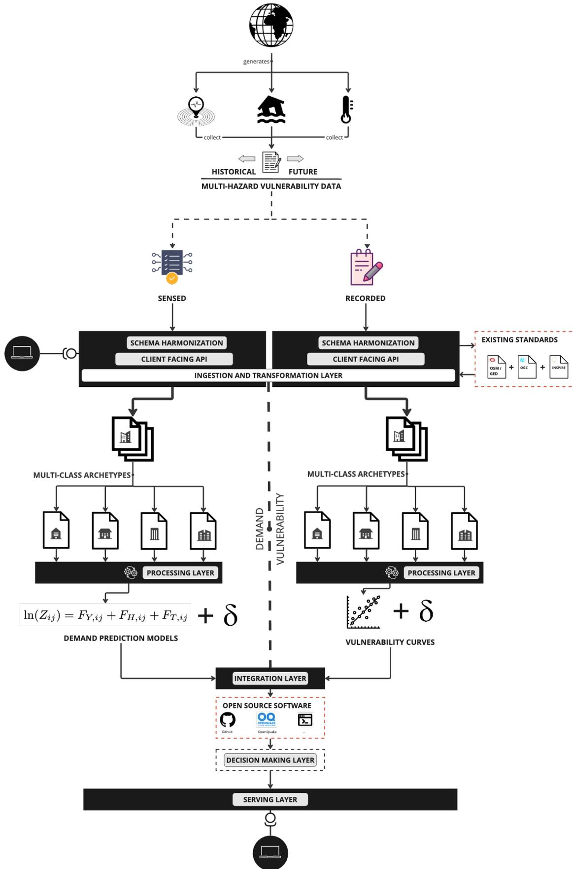
Fig. 6. Schematic pipeline for the digital tools supporting the vulnerability database.
