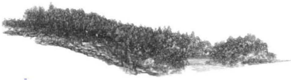
Figure 3.8: Captured image of the intensity visualization. Each voxel is assigned a transparency value based on its average intensity. The model has been made by Christopher Wood source: (Pyyssalo et al., 2009)
