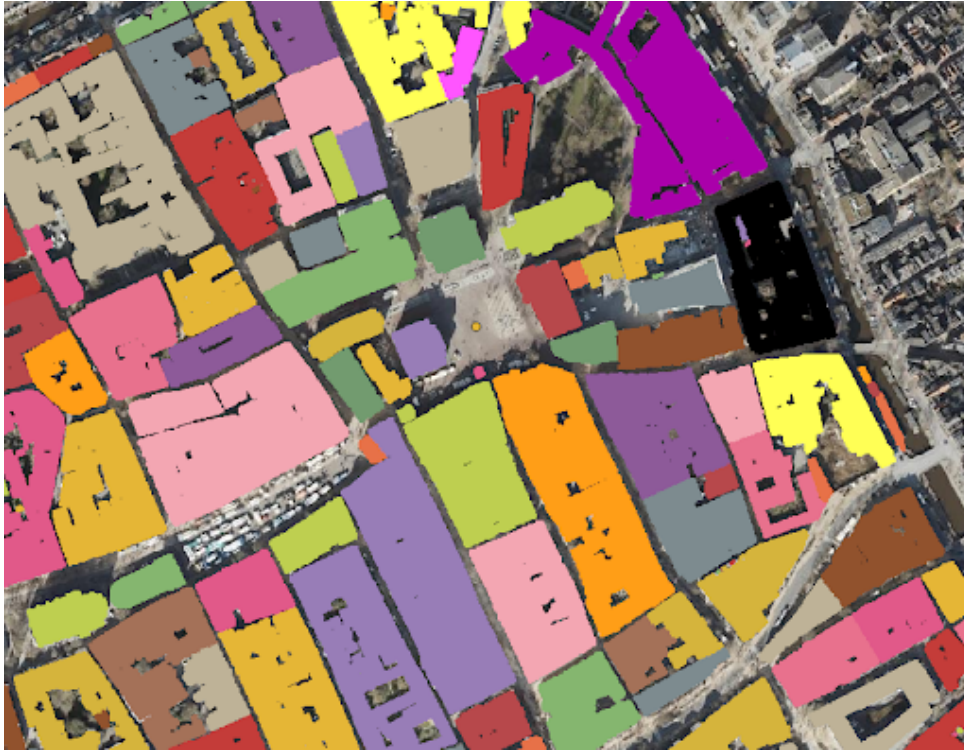
Figure 4.8: Roof points clustered into distinct building footprints using the DBSCAN algorithm, represented by alternating colors.
