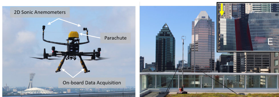
Figure 2.1: Equipments to collect real world wind data, (left) a drone with 2D sonic anemometers, (right) a 3D sonic anemometer on the top of a building. (sources: [56])
